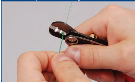
1.4 Strip Off Coating
